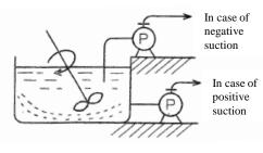
② To install pipe in simple manner Both suction and delievery pipes should be installed in simple manner without bend and reduction/expansion so that clogging of particle matter or holing by wear could be prevented. ③ To use valve as little as possible Do not use sluice valve ect. to regulate capacity. It will cause to shortage of life by wear and result in block in the piping. When valve is installed in case of slurry, it could be used for shut-down for disassembly/assembly.
