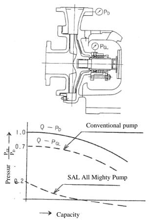
$P_D$  Pump discharge pressure  $P_{GL}$  Discahrge pressure at gland during opeartion (reduced pressure by rear impeller vane) ■ Features on materials (refer to P6 Q1 and P9 Materials of main parts)
