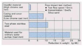
• For impeller which needs most wear resistance, high chrome casting (EBAREX-H) ,which is by far the best in wear resistance, is used. (approx. 20 times of conventional cast iron in wear resistance)
