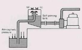
Even when the pump is stopped, all water in the tank will not drain which means it is
