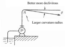
Countermeasure in case of excessive capacity.
