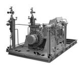
Centerline support, Radial split Double Volute casing Double suction impeller Full compliance with API 610 Pull Out Design of rotating assembly Low NPSH performance
